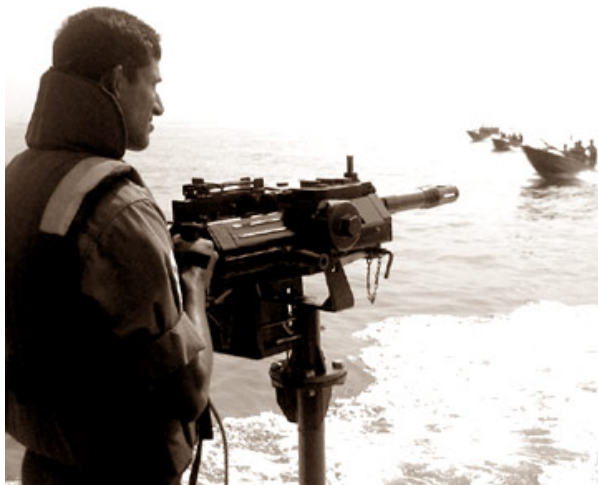
Singapore Technologies Kinetics' Automatic Grenade Launcher has provided the inshore patrol craft with increased firepower to engage Sea Tiger attack craft, particularly suicide boats.
